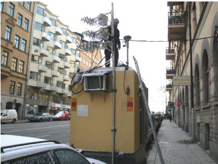
Figure 4.3.2 The 48 sampling heads for the campaign sampling of PM 10 , PM 2.5 and PM 1 at Hornsgatan in Stockholm.
