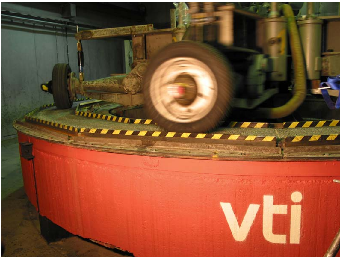
Figure 3.1.1 The VTI circular road simulator.
