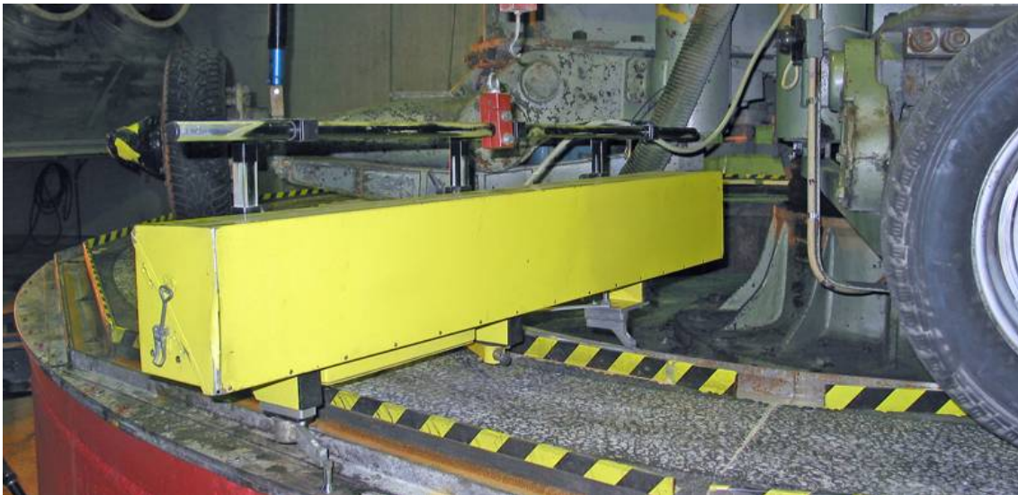
Figure 3.1.2 Laser profilometer applied to the road simulator.
