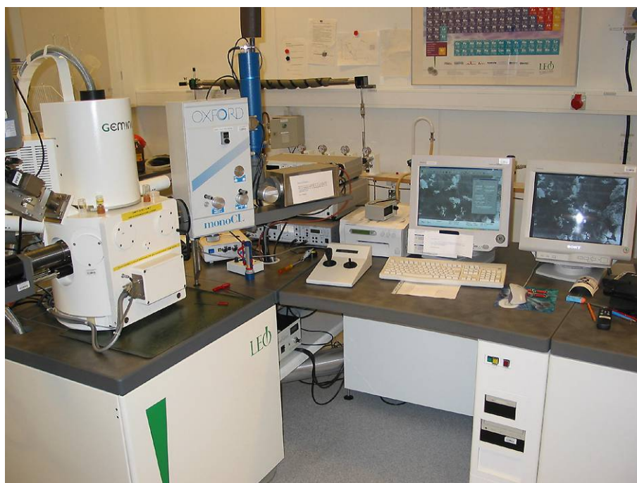
Figure 3.3.1 SEM (scanning electron microscope, LEO Gemini 1550) equipped with EDX (emission dispersive x-ray spectroscopy, Link ISIS) at the Institution of thin film technique at Linköping University.
