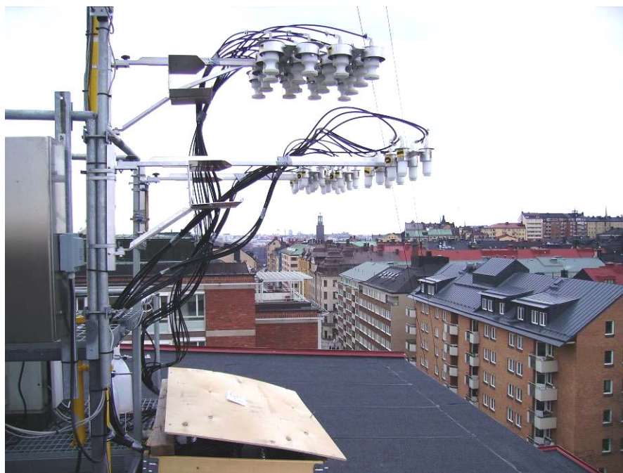
Figure 4.3.3 Sampling heads for the campaign sampling of PM 10 , PM 2.5 and PM 1 at roof level at Torkel Knutssonsgatan in Stockholm.
