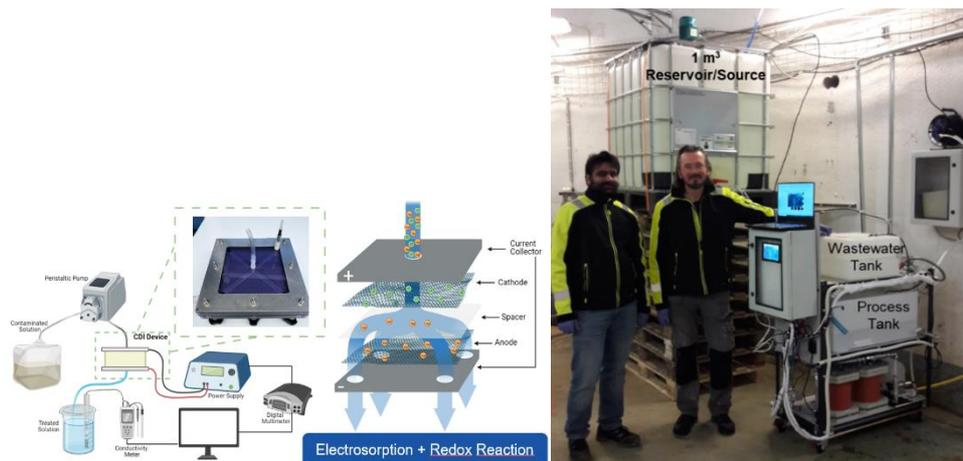
**Fig. 2.** CDI-modules used in the tests: left – lab scale device; right – pilot-scale plant with two CORE® CDI modules.
