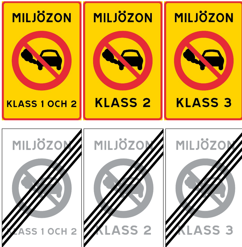
Figure 2 Swedish road signs for LEZ, class 1 and 2, entering and exiting the zone (The Swedish Transport Agency, 2020).
